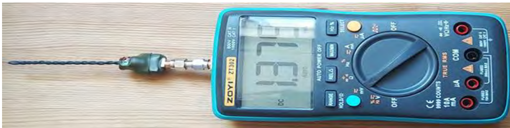
Fig. 1. Avsharov's meter built on a straight bifilar antenna
